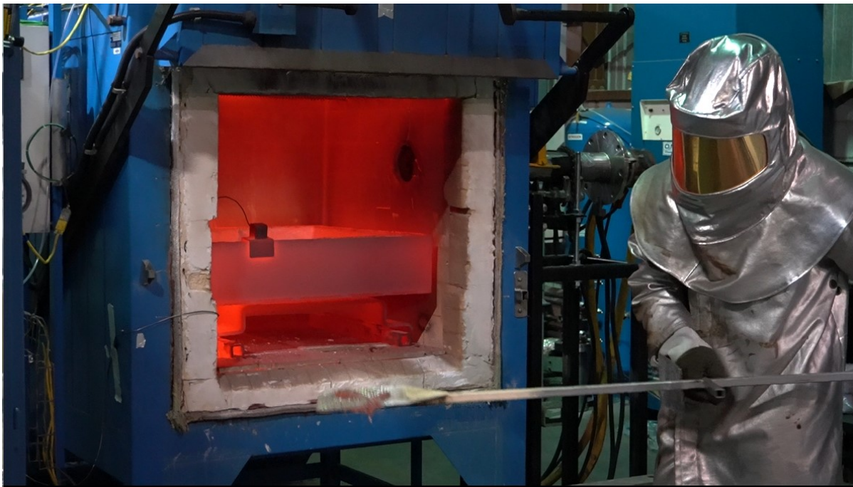
Figure 1: An engineer removes metal from a furnace during PyroGenesis' tests using plasma torches within an aluminum melting furnace supplied by its client Constellium.
