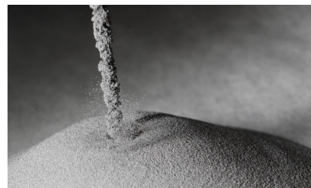
PyroGenesis' titanium metal powder as produced by its NexGen™ plasma atomization system
