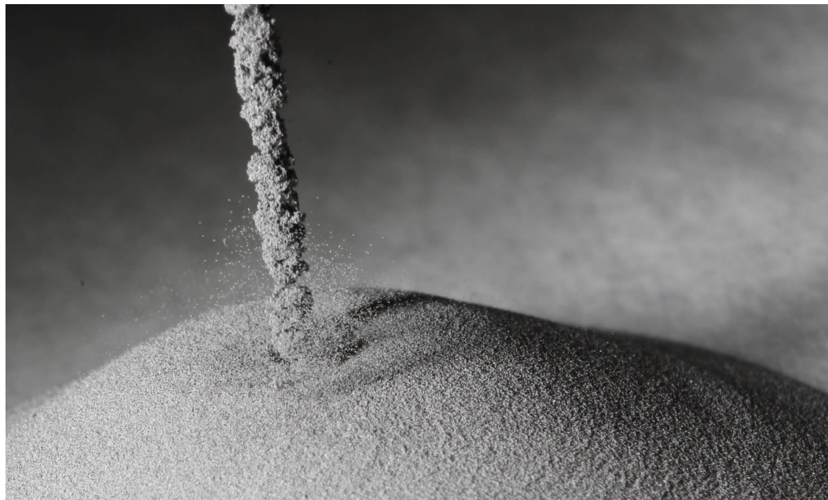
Image: PyroGenesis' titanium metal powder as produced by its NexGen™ plasma atomization system.
