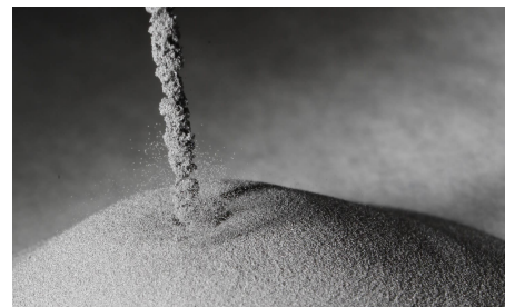
PyroGenesis' titanium metal powder as produced by its NexGen TM plasma atomization system.
