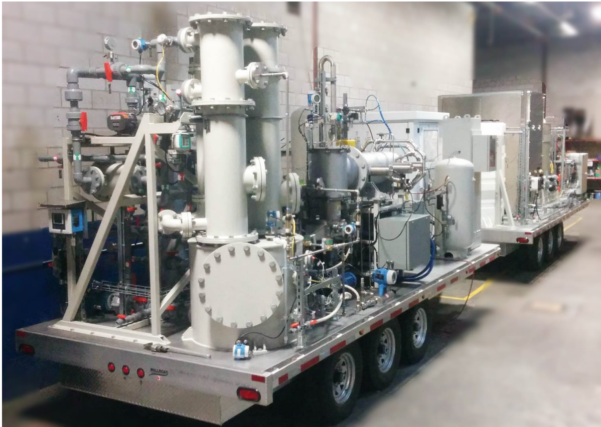
Image: a mobile version of PyroGenesis' PACWADS system for use in destroying chemical weapons.
