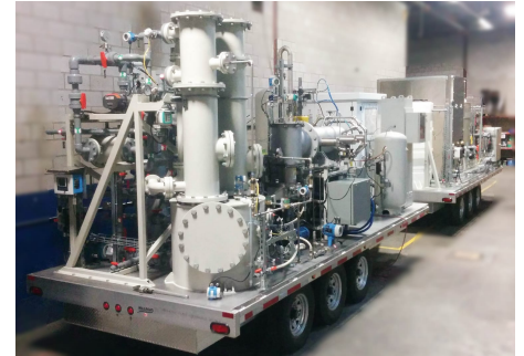
A mobile version of PyroGenesis' PACWADS system for use in destroying chemical weapons.
