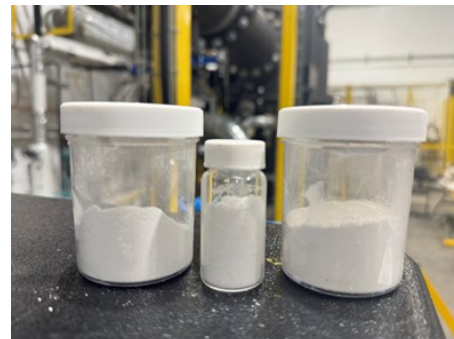
Fumed silica, produced by the fumed silica reactor
