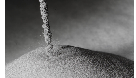
PyroGenesis' titanium metal powder as produced by its NexGen™ plasma atomization system.
