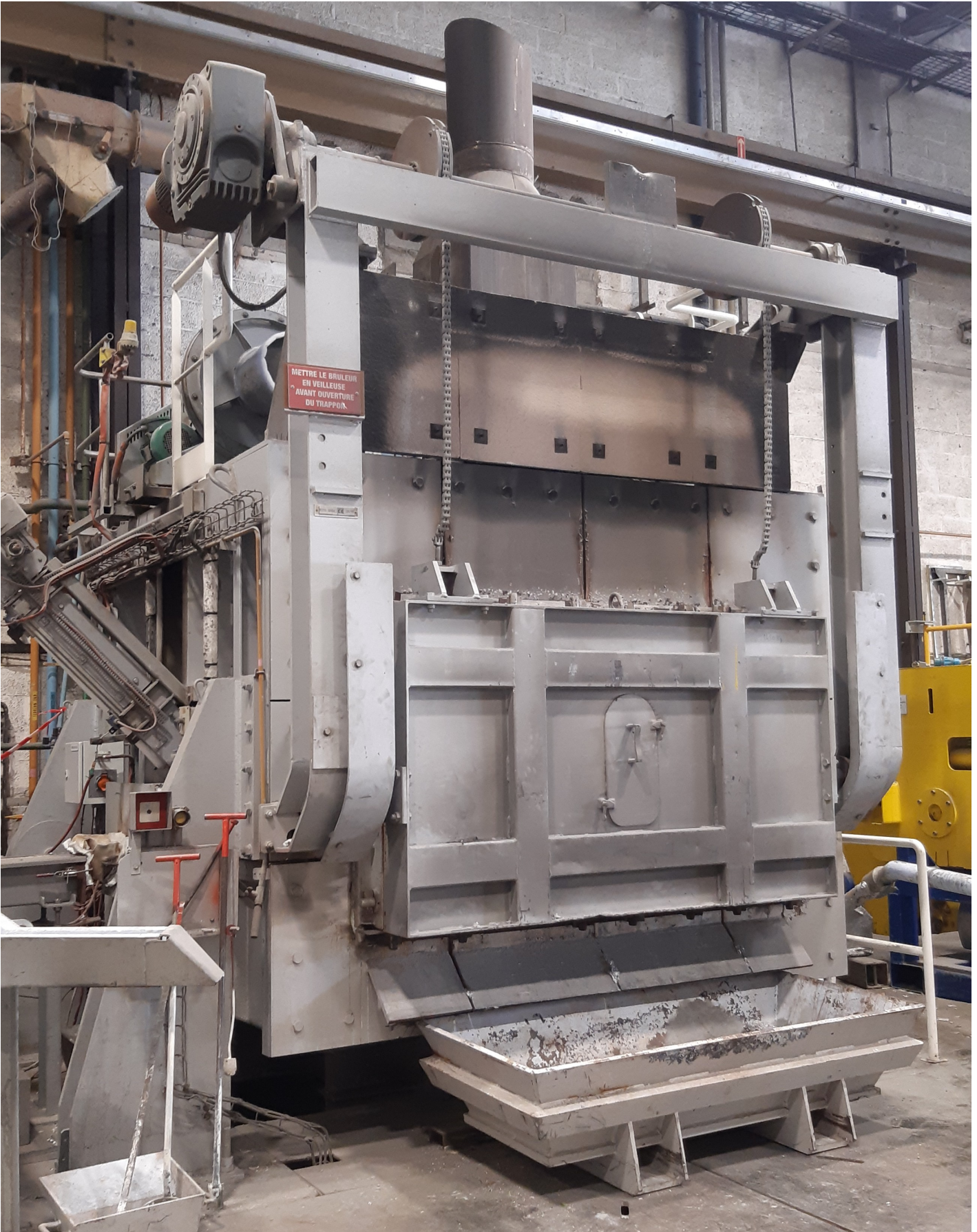
Image: secondary melting furnace in use at one of Constellation's aluminum facilities. Photo courtesy of Constellation.
