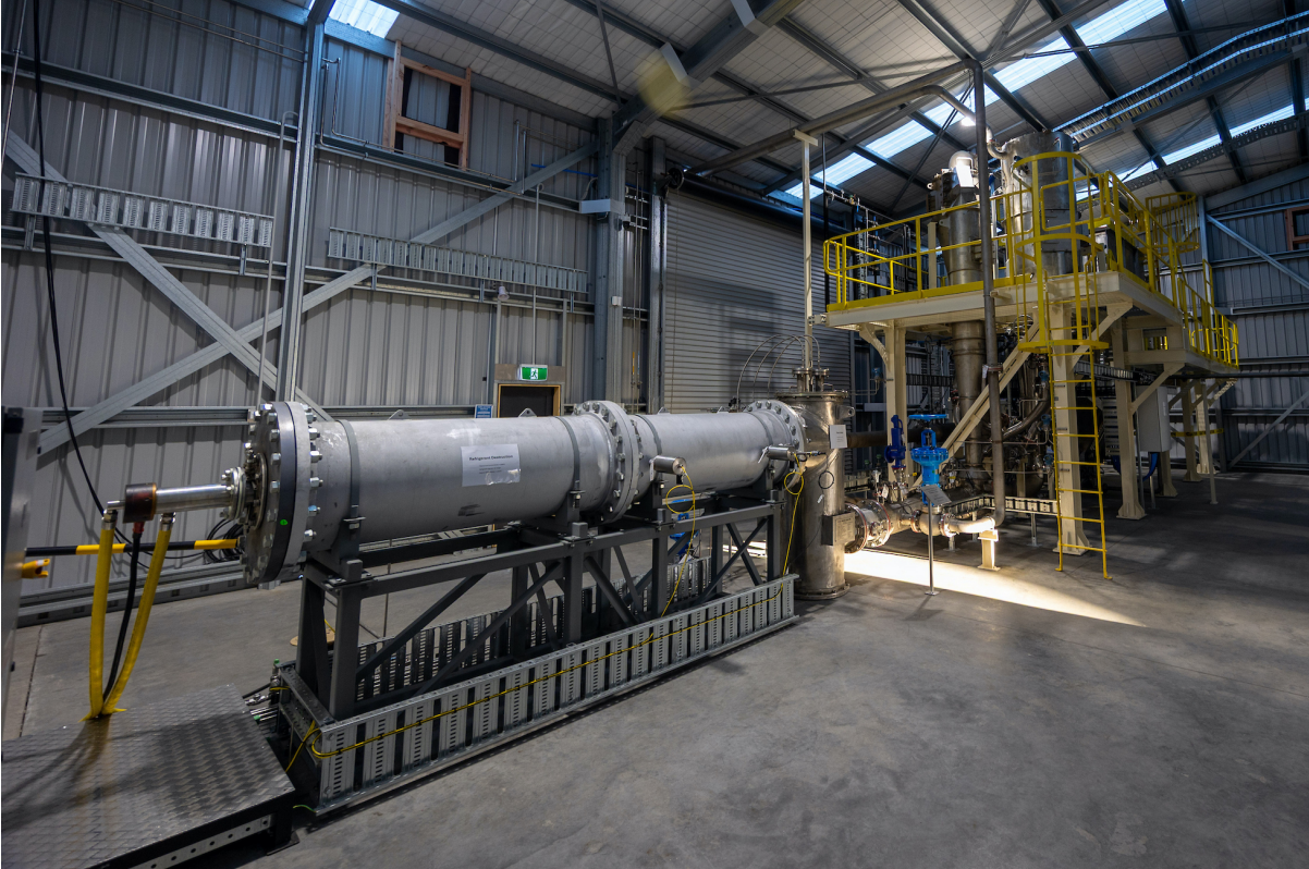
Image 1: PyroGenesis' steam plasma arc (SPARC™) hazardous refrigerant destruction system, shown at the opening of New Zealand's National Refrigerant Destruction Facility. Photo Credit: Jamie Troughton/Dscribe Media.
