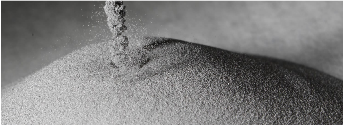
Image: PyroGenesis' titanium metal powder as produced by its NexGen™ plasma atomization system.
